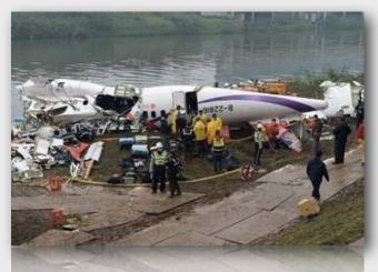
Forty-three of the 58 people on board were killed when the ATR struck a bridge and crashed into the river below in February 2015. The council's report said an inconsistent electrical signal in the No. 2 engine's auto-feather unit likely caused an uncommanded feathering, which started the accident sequence.
